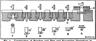
Fig. 5. Construction of Punches and Dies and Successive Operations in Drawing and Piercing Shell F
